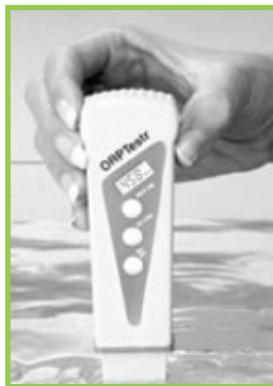
**Hand-Held Meters:** Typically low cost, fit in the pocket and are very portable. Both meter and electrode are integrated together into a compact design. Useful life of the electrode is 1 to 2 years. Calibration testing and cleaning is recommended at least once a week to ensure ongoing reliability. This type of meter can also come with a pH electrode as well.
